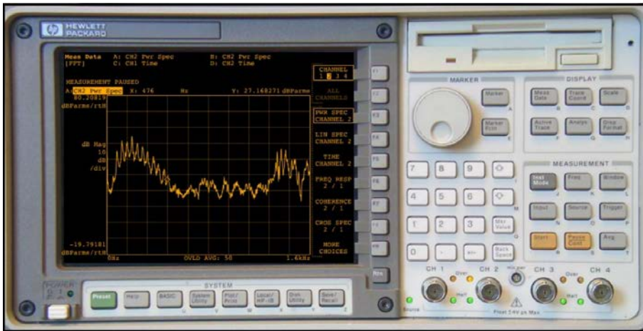
Figure 21. Screen shot of the signal analyzer when PSD of a random sound is plotted using the VISIR acoustic lab.
