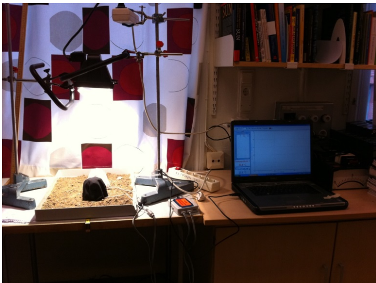
Figure 1. Experiment collecting temperature of one white and one black object. In the diagram, on the computer screen, the temperature of the two objects is displayed as a function of time.
